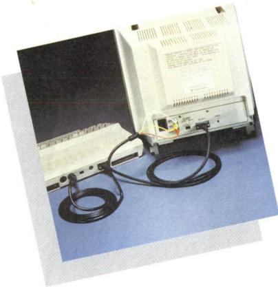
Note that you can connect a composite monitor and an RGBI monitor to the Commodore 128 at the same time. This allows you to switch between 40 and 80 column displays.
