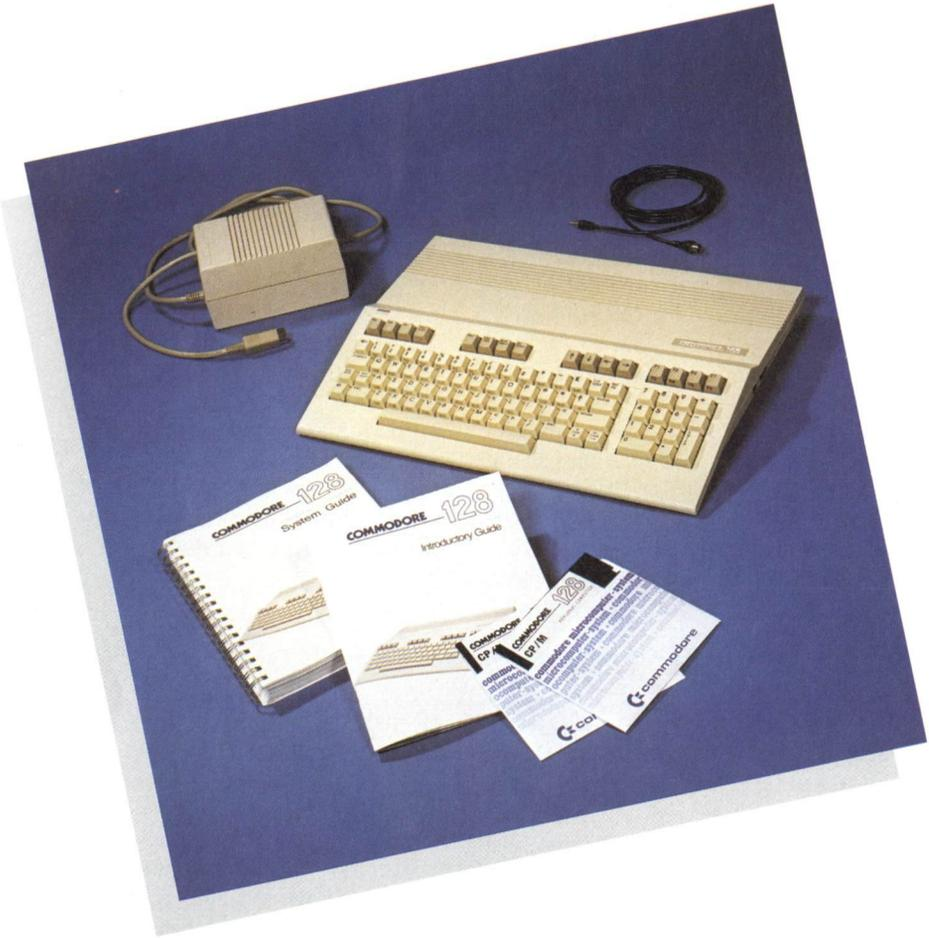
The Commodore 128 Personal Computer is supplied in one box which contains the Commodore 128 Personal Computer itself, its power supply, an RF lead, two manuals (this Introductory Guide and the Systems Guide) and the CP/M Systems Disk.
