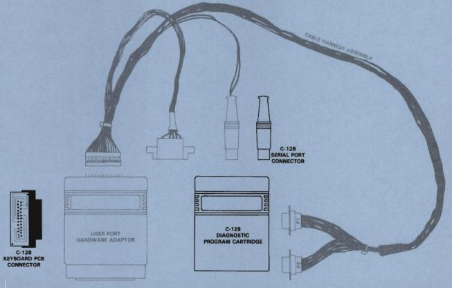
The User Port Hardware Adapter and Cable Harness Assembly (gray shaded assemblies) used with the C128 Diagnostic are the same as used with the C64 Diagnostic with the exception of the Keyboard Connector PCB and the Serial Port Connector (black outlined assemblies).
