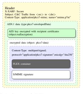
Fig. 1. Components of a FLEX message
