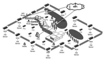
Fig 2. WSN prototype deployment diagram. The three major objectives of the system are shown: surveillance, multi-tracking and critical monitoring.
