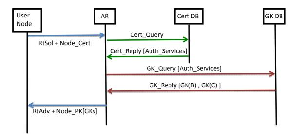
Figure 1: Messages exchange on the LAN side interface
