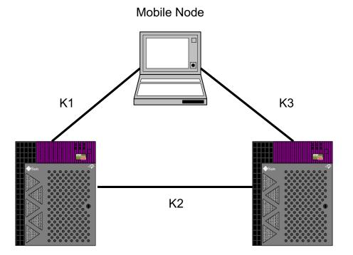
When the keysets are distributed, the Mobile IP messages are authenticated using the new keys.
